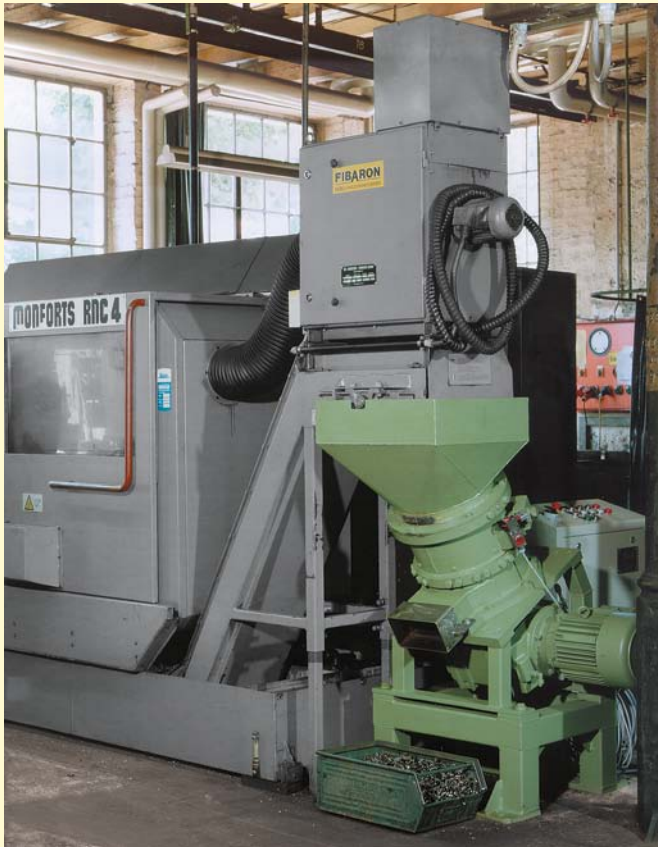
The swarf crusher RS 300 K on the photo (green) is directly filled by the drag-out conveyor of an NC-processing machine.
