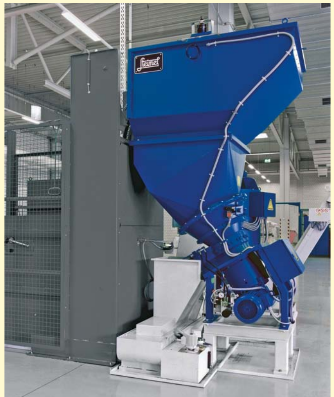
Swarf crusher RS 300 E in a swarf processing plant consisting of a lifting and tipping unit, swarf crusher RS 300 E, scraper conveyor, a Type Permolux-Polar K 51 centrifuge and a second scraper conveyor having a swivelling discharge chute to discharge the crushed swarf into the customer's containers.
